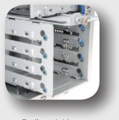
Optional 4-bay 3.5" HDD cage with anti-vibration absorbers
